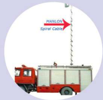
Lighting Mast Cable
